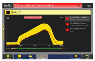
The optional PTO Replay feature brings single functions of the Process Tracking Office (PTO) directly to the device. This function allows the operator to analyze process error curves and their progression through a replay function.
